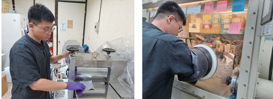
Button Cell Fabrication Process: Coating the battery slurry, followed by rolling to form electrode sheets, and final assembly.
